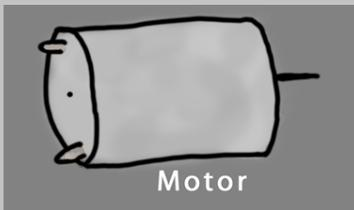
A motor converts electrical energy into mechanical energy or motion. They do not have polarity, but switching red and black will reverse the motor's direction. We have found that motors used for Squishy Circuits should have terminals attached and a low current rating (~30mA or .030 Amps).
